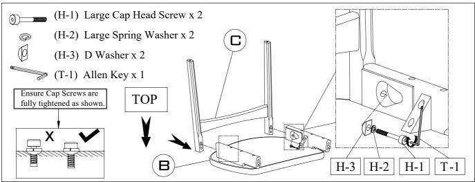
Position Seat (B) upside down onto a padded, no-marring surface. Position Front Frames (C) onto the front of Seat (B) as shown. Insert Large Cap Head Screw (H-1), Large Spring Washer (H-2) and D Washer (H-3), through the holes in each Seat (B)'s frame into the receiving holes on the Front Frame (C), arrange the hardware in the order as shown. Do not yet fully tighten Bolts.
