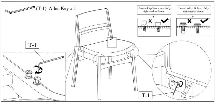
After verifying that all four legs have settled properly (in Step 3), fully tighten all bolts and cap screws from Step 1-2 using Allen Key (T-1). DO NOT use a power drill or overtighten any of the bolt hardware as this may damage the assembly.
