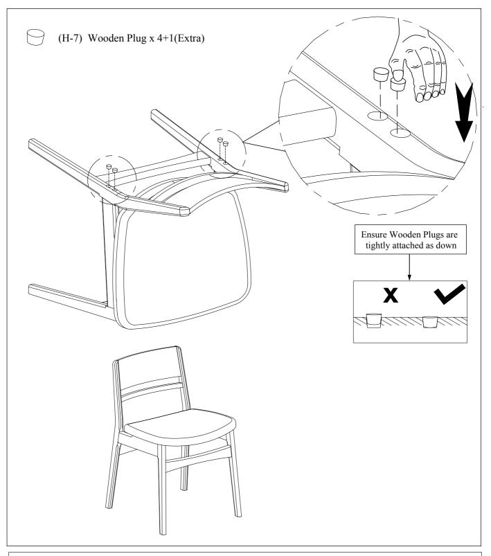
Use your hand to press Wooden Plug (H-7) into the holes in Back Rest as shown. One extra Wooden Plug (H-7) is provided. Assembly is now complete and the product is ready for use. NOTE: Hardware may loosen over time. Periodically check that all connections remain tight and adjust as needed.
