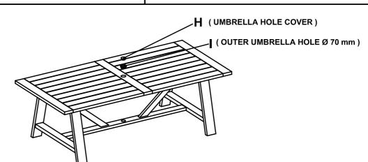
Turn the table to upright position. Install the umbrella hole cover (H), and outer umbrella (I) into the hole of table top (A) as shown in the diagram.
