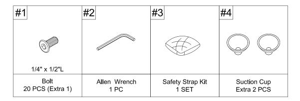
Step 1. Insert cross bars (part G) to front shelf bar (part E) and back shelf bar (part F) using bolts (part #1) and allen wrench (part #2).
