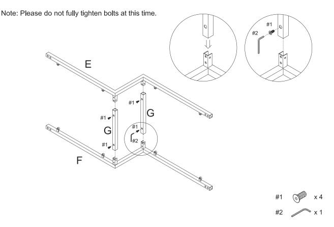
Step 2. Insert top front bar (part C), top back bar (part D) assembled unit (parts E, F & G) to left frame (part A) using bolts (part #1) and allen wrench (part #2).
