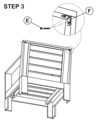
Install Elbow hardware (F) to the top corners where the backrest (B) meet side frames (A1 & A2). Insert all 1/2" bolts (E) into each hole and then tighten the bolt using screwdriver.
