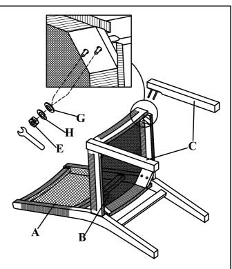
Attach the seat (B) to Back rest (A). Ensure the seat (B) align to the matching holes. Insert the small washer (F), spring washer (H) and 2" bolts (D) to the Attach the legs (C) into the seat (B). Secure it with big holes as shown in the diagram above. Adjust the bolts washer (G), spring washer (H) and nut (E). to the right position before screwing. Do not fully tighten the bolts yet.
